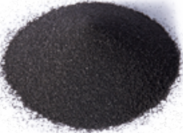
SEPARATOR SAND Separator sand prevents strip tiles from sticking together during production.
