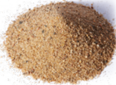
SEPARATOR SAND Separator sand prevents strip tiles from sticking together during production.
